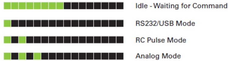
FIGURE 10. Normal Operation Flashing Patterns
