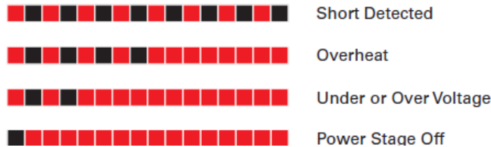
FIGURE 11. Exception or Fault Flashing Patterns
