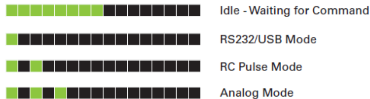
FIGURE 8. Normal Operation Flashing Patterns
